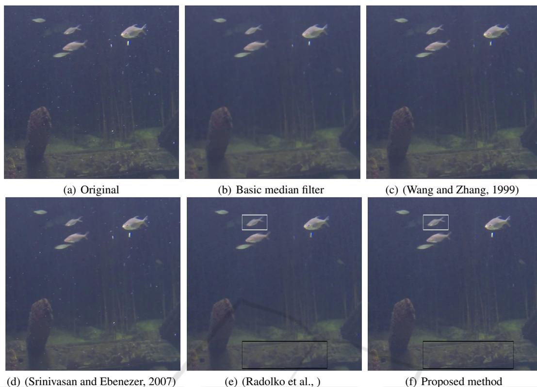
Figure 4: The original image (a) and results after applying basic median filter (b), (Wang and Zhang, 1999) (c), (Srinivasan and Ebenezer, 2007) (d), (Radolko et al., ) (e) and our proposed method (f). Areas assigned with rectangles shows how (Radolko et al., ), (Banerjee et al., 2014) smoothed the true edges of the image details which are preserved in proposed method.
