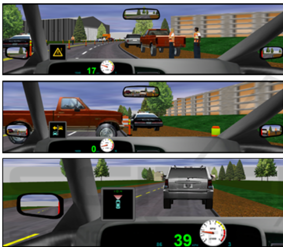
Figure 3: An alarm is showed in the HCI interface of the driving simulator.
