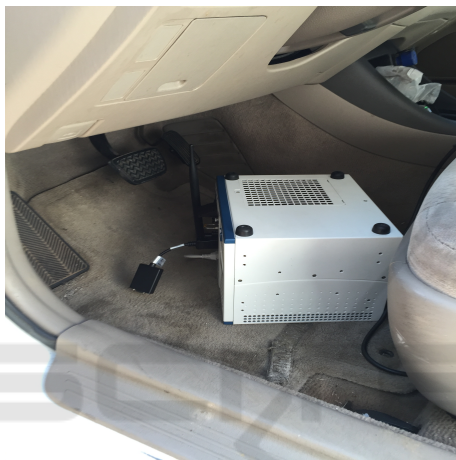
Figure 16: VSA position in the driver's footwell in Toyota.
