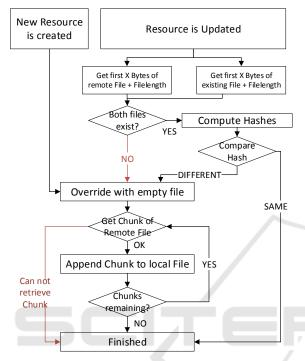
Figure 2: Upload of new or updated Resources to the HDFS through the Plugin. Possible occurring errors are shown in red.
