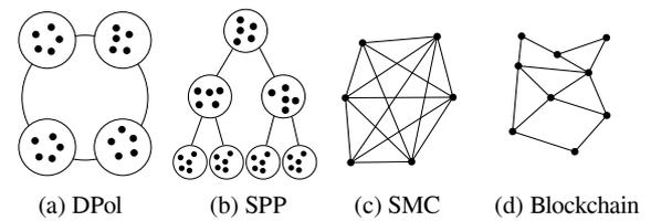
Figure 2: Topology of distributed voting protocols. (a) DPol and (b) SPP have a higher degree of hierarchy than (c) SMC and (d) blockchain-based protocols due to partition of voters in clusters. This way, the number of exchanged messages can be reduced at the cost of less equipotent voters with less flexible roles. Unstructured SMC- and blockchain-based protocols use a distributed topology allowing for equipotent voters.
