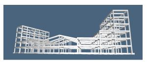
Figure 7: A spatial concrete frame generated, from a small .csv file, by the pyplasm plugin spatialFrame.
