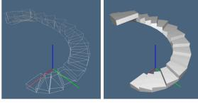
Figure 6: (a) The generating function of a strongly parameterized spiralStair; (b) default spiralStair.
