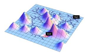
Figure 4: TRRT exploration in an artificial environment with many high cost areas.
