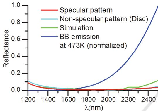
Figure 3: Reflectance curves measured and simulated for the highly emissive produced patterns, and normalized black body emission at 473K.
