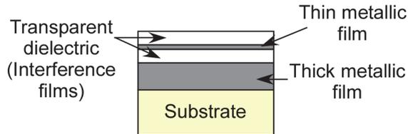
Figure 1: Multilayer structure of high emissivity patterns.
