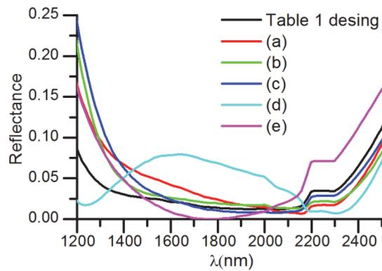
Figure 4: Simulated reflectance spectra for coatings with different thicknesses: multilayer structure as described in Table 1 (black line), (a) Outer transparent dielectric layer with a 10% thicker thickness than in Table 1, (b) both dielectric layers with a 10% thicker thickness, (c) All layers with a 10% thicker thickness, (d) Thin metallic film with a 30% thinner thickness, (e) Thin metallic film with a 30% thicker thickness.
