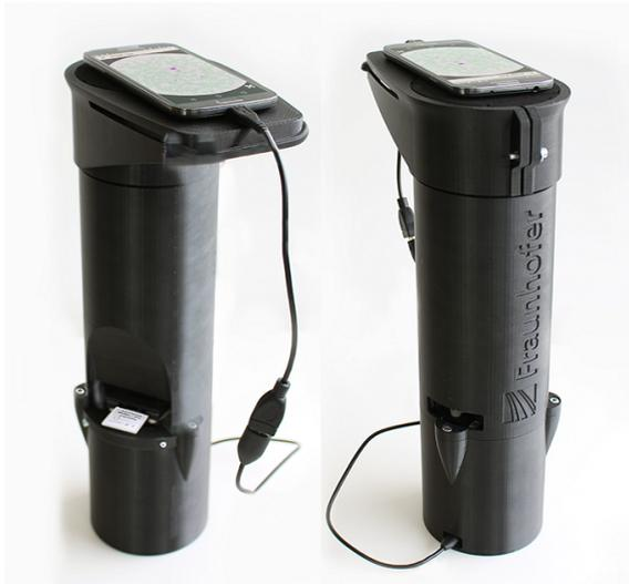
Figure 1:  $\mu$ SmartScope with smartphone attached and malaria-infected blood smear inserted.
