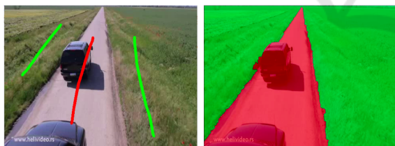
Figure 4: On the left, the first frame of a video sequence, where some seeds or markers have been defined for the road (red) and other (green) classes. On the right, the segmented image using the watershed technique with the defined markers.
