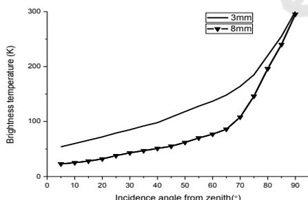
Figure 2: Brightness temperature of sky at the various angles of relatively zenith.
