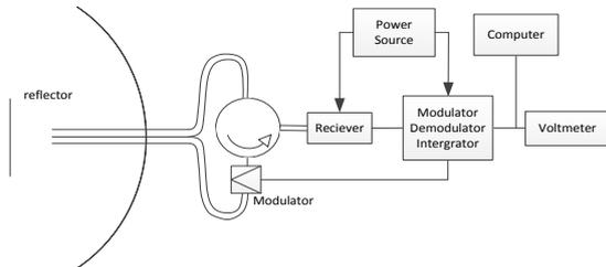
Figure 8: Block-scheme of the simplest 8 mm microwawe discriminator.
