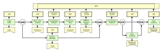
Figure 7: Example process with RFID support.
