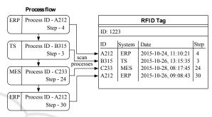
Figure 3: Data structure on the RFID tag after scanning.
