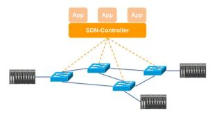
Figure 1: In SDN the network devices (middle) forward network flows programmed by a SDN controller (top) between end-devices (left/right). The SDN controller could also be integrated into one of the end-devices.
