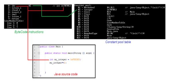
Figure 4: example of java class file (bytecode) from java source code.
