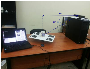
Figure 3: The 3D acquisition system contains: Kinect camera, RGBDemo software and rotating support commanded by arduino Kit.
