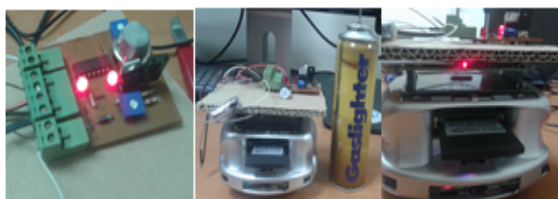
Figure 7: Gas sensor circuit combined with khepera III.
