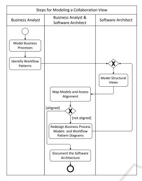
Figure 4: A process diagram representing the process of modeling a collaboration view.
