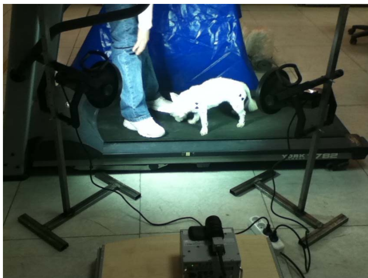
Figure 3: Experimental set-up for recording a dog's walking behavior.
