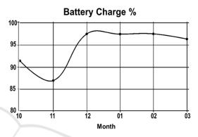
Figure 9: Average charge percentage graph of a node's battery with solar cell during 5 months.
