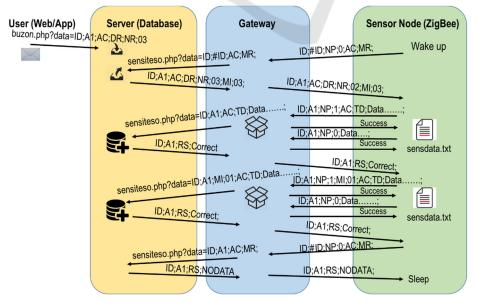
Figure 5: Time chart example of the communication protocol.
