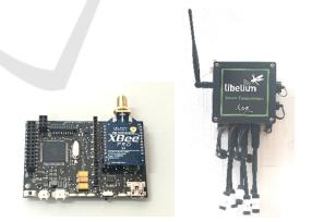
Figure 3: The Waspmote OEM version, left, and the Plug&Sense! Version, right.
