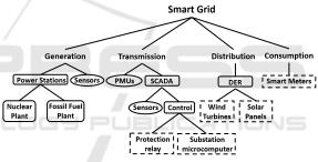
Figure 3: Devices in the smart grid domain.
