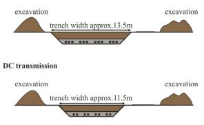
Figure 3: Exemplary trench width for power-cable transmission (Hofmann, 2015).
