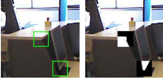
Figure 2: Projection of features s_0 and s_1 on the image \mathcal{K} = s_0.\mathcal{J} = s_1.\mathcal{J} , showing their bounding rectangles s_0.R, s_1.R (left) and their masks s_0.\mathcal{M}, s_1.\mathcal{M} (right).
