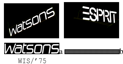
Figure 10: OCR recognition failures due to (a) challenging font, (b) small text size and (c) complex design: original image (top), text rectification result (middle) and OCR transcription using Tesseract (bottom).
