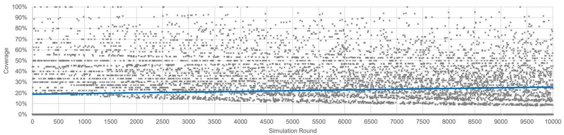
Figure 5: Distribution of city network supply coverage. The rounds on the x-axis are sorted ascendingly with respect to the city network size. This result shows higher ratios of coverage with growing network sizes on average, as more nodes contribute to a more coarse-grained distribution and promote the chances of valid Holon setups.
