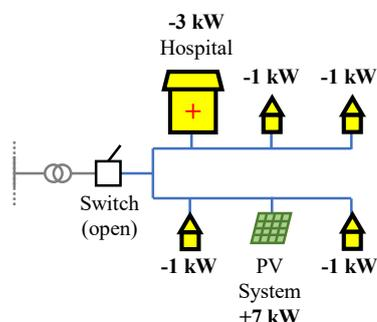
Figure 3: A micro grid in islanded operation.
