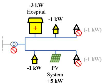
Figure 2: A disconnected city network is partly supplied by a local PV system.
