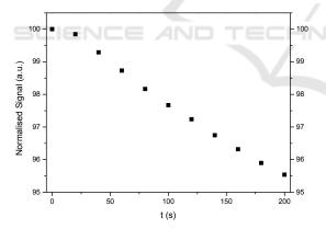
Figure 6: Quenching profile of PFO exposed to DNB vapour in nitrogen.
