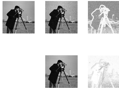
Figure 1: From left to right top to bottom: Original image; Image affected by additive gaussian noise; pointwise SSIM map; Image affected by gaussian blur; pointwise SSIM map.
