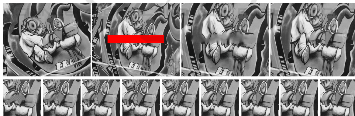
Figure 7: First row: source image, target image with the inpainting domain shown in red, and close-ups around the inpainting area of the NL-Means result and the result of our method. Second row: evolution of the inpainting domain over iterations of our method (every third iteration).
