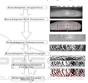
Figure 3: Overall architecture of FKP recognition system.
