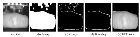
Figure 5: Steps involved in Knuckle Area Detection.
