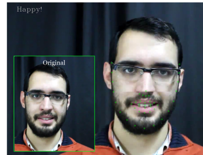
Figure 10: VR Assessing Facial Expressions: Correct Emotion Recognition result (blue) and no Expression Predictor result, since there is not movement. Check original image in green box.
