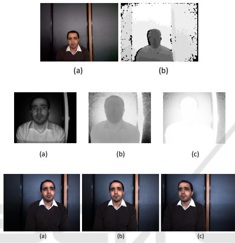
Figure 1: Top row: example of infrared sensor images (Kinect): (a) color image (b) depth image. Middle row: example of TOF sensor images (SR4000): (a) infrared image (b) depth image (c) confidence matrix (bright pixels show high confidence). Bottom row: example of image triple acquired with the stereo camera (Bumblebee XB3).
