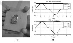
Figure 5: (a) AREM Gateway on a Vicon frame, (b) Roll orientation comparison with Vicon.
