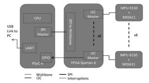
Figure 1: Centralized embedded motion system synopsys.
