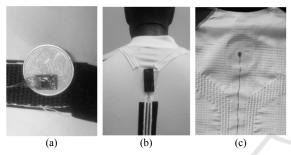
Figure 3: (a) New MPU9250 tags with thin wires, (b)(c) Sensors tags integrated into a t-shirt.
