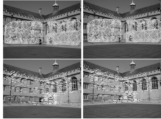
Figure 4: The top row visualize the delaunay triangulation of the points. The bottom row shows reconstructed surface normals using homography of large walls on sequence 'College'.
