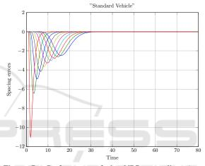
Figure 7: Performance of the NRP controllers ( $\tau = 0.5s$ ,  $L_{des} = 40m$ , h = 1.3s, k = 4,  $\lambda = 0.4$ ). The different lines correspond to the spacing errors of each NRP controlled vehicle in the stream.
