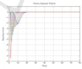
Figure 8: Performance of the Pareto optimal controllers  $(\tau = 0.5s, L_{des} = 40m, h = 0.9s, k = 10, \lambda = 1.6)$ . The different lines correspond to the spacing errors of each Pareto optimal vehicle in the stream.
