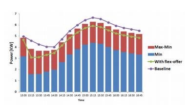
Fig. 12. Example of load shedding implemented using FlexOffers compared to estimated baseline.
