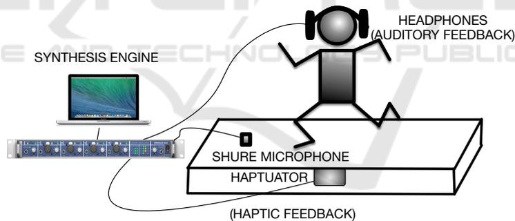
**Fig. 6.** A visualization of the setup used in the studies following the NIW project. It clarifies the placement of the actuator. We can see that feedback was presented through headphones connected to synthesis engine describe in the previous section via Fireface 800 sound card [35].
