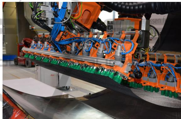
Figure 2: Both robots gripping a cutpiece.
