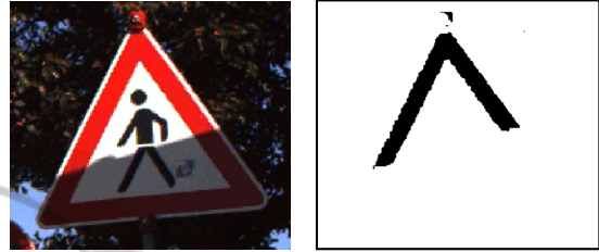
Figure 2: Example of color extraction in RGB.
