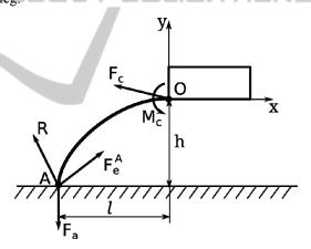
Figure 3: Forces and torques acting on the robot's leg.
