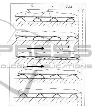
Figure 8: Mode of motion of the mobile microrobot along a flat surface.
