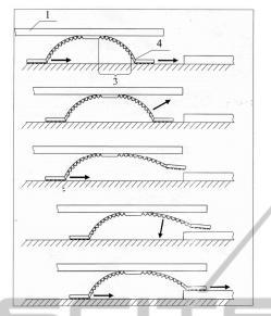
Figure 9: Mode of motion of the mobile microrobot along a stepped surface.
