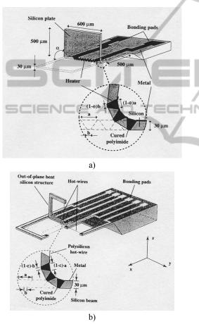
Figure 1: View of MEMS polyimide joint structure (Ebefors 1999). a) MEMS triple hot-wire; b) Isometric view of a three-dimensioned structure based on polyimide joint with three V-grooves.
