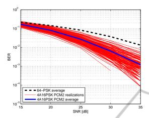
Figure 1: BER versus SNR results for "Parking on Land" scenario.
