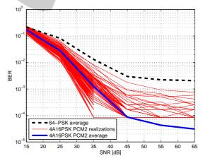
Figure 4: BER versus SNR results for "Flying Platform" scenario ( $f_0 = 4 \ GHz$ ).
