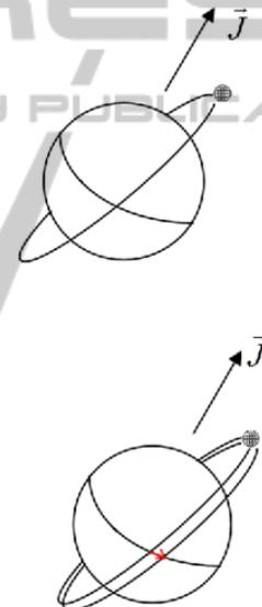
Figure 2: Orbital planes in a reference frame fixed with respect to distant stars. (Top) classical mechanics; (bottom) general relativity. The red arrow shows the Lense-Thirring nodal shift.
