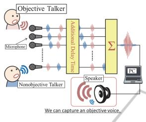
Figure 4: Schematic of the DSBF method.
