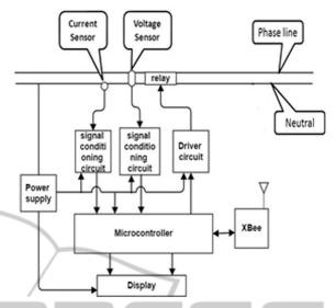
Figure 3: Hardware architecture of an intelligent module.
