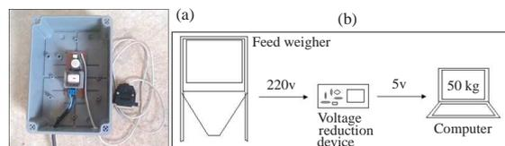
Figure 2: Device for voltage reduction.
