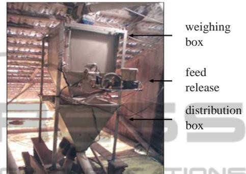
Figure 1: Mechanism for weighing feed.
