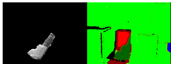
Figure 3: Experiment without the second step of the sliding reduction. The object tilts to the right side.
