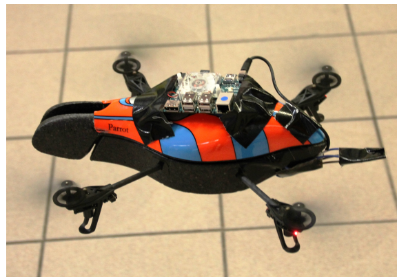
Figure 1: Parrot AR Drone carrying an Odroid hardware platform for real-time vision processing.
