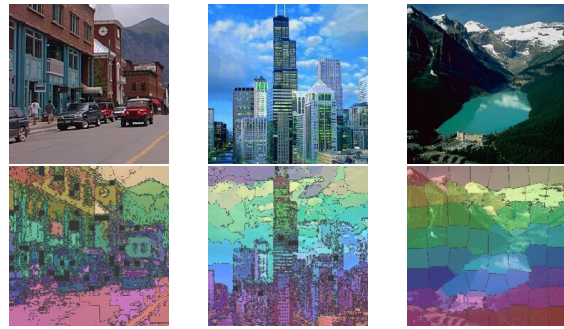
Figure 4: Visualization of the SLIC algorithm on three images of the SIFT Flow database. The parameters are set to K = 60 and w_s = 1 ; w_s = 10 ; w_s = 50 (from left to right).
