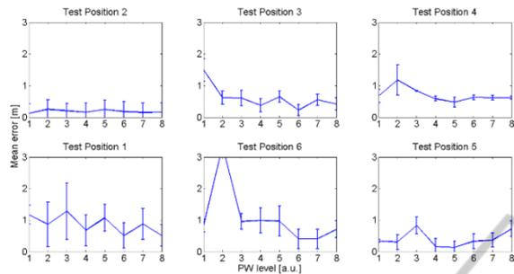
Figure 5: Mean positioning error and its standard deviation calculated on 100 measurement performed for each position are shown as function of the different power levels.
