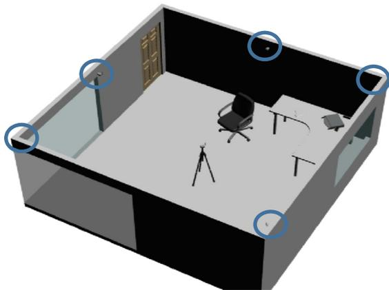
Figure 1: Schematic representation of the test room arrangement. It is possible to note the mobile node on a tripod and the anchors node attached on the walls highlighted by the circles.
