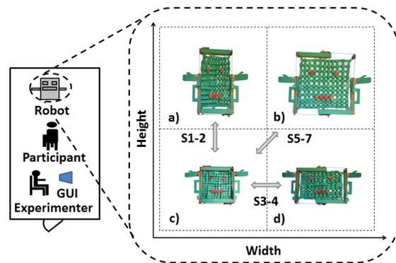
Figure 4: Experiment layout and depiction of the seven size changes which participants observed (S1-7) using actual photos of our prototype, Suica, changing between four states: (a) tall, (b) large, (c) small, and (d) wide.
