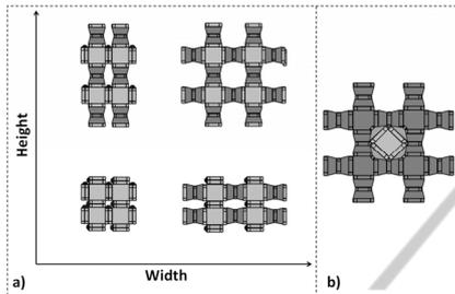
Figure 2: Size-changing cover: (a) a main layer which enables changes in height and width, and (b) an optional top layer (shown lightly shaded over the dark main layer).
