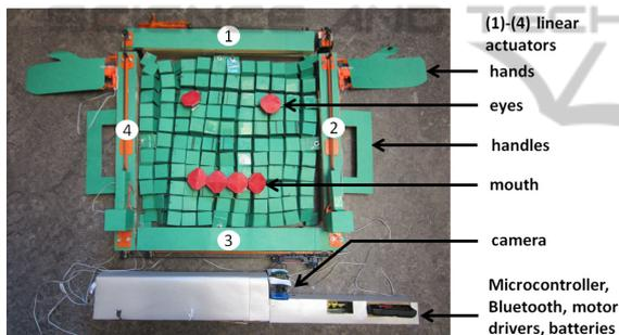
Figure 3: Actual photo of our humanoid prototype, Suica, indicating component locations.
