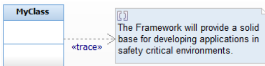
Figure 4: A class inside Rhapsody, which is linked to a representation of a requirement from Polarion.
