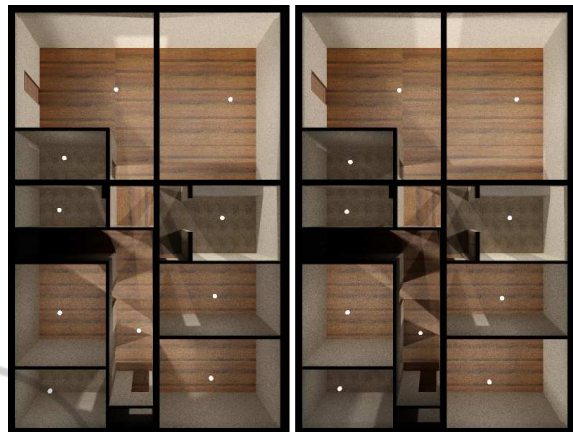
Figure 6: Correctness experiment. Left: the user defined light sources, whose irradiance to sampling points is measured and used as a goal. Right: the computed light configuration produced by our algorithm (4.3% error).
